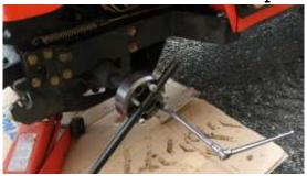
H. Get your socket & add Locktite to the studs on the spacer. Install the rim/wheel & now use the new nuts from the spacer, making sure they are flip to the proper end. Torque the nuts to 90 ft. lbs for the rim in the same 3 steps as above (3/4" Socket).
